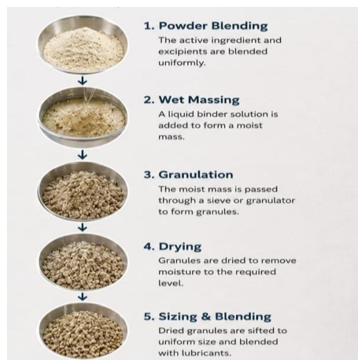
Fig. 2.3 Wet Granulation method
