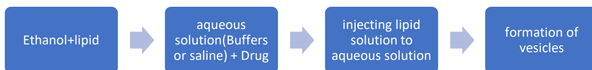
Fig. 5: Preparation of Liposome by Ethanol Injection method.
