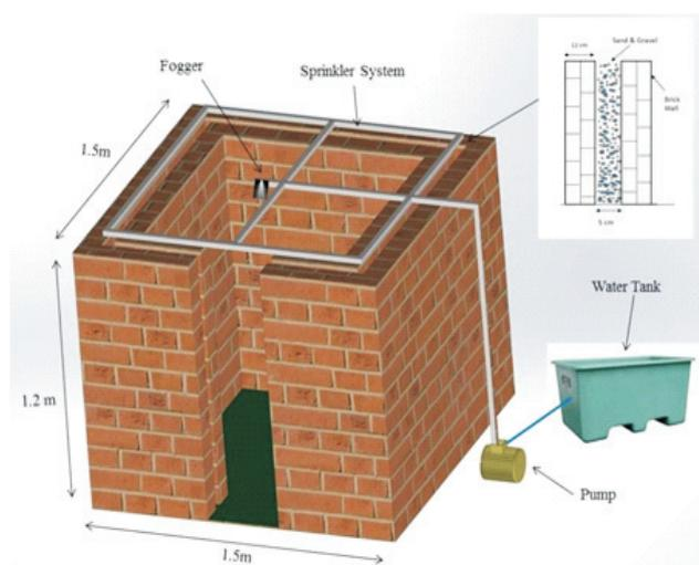
Figure 1: Experimental set up of evaporative cool hydroponic chamber
