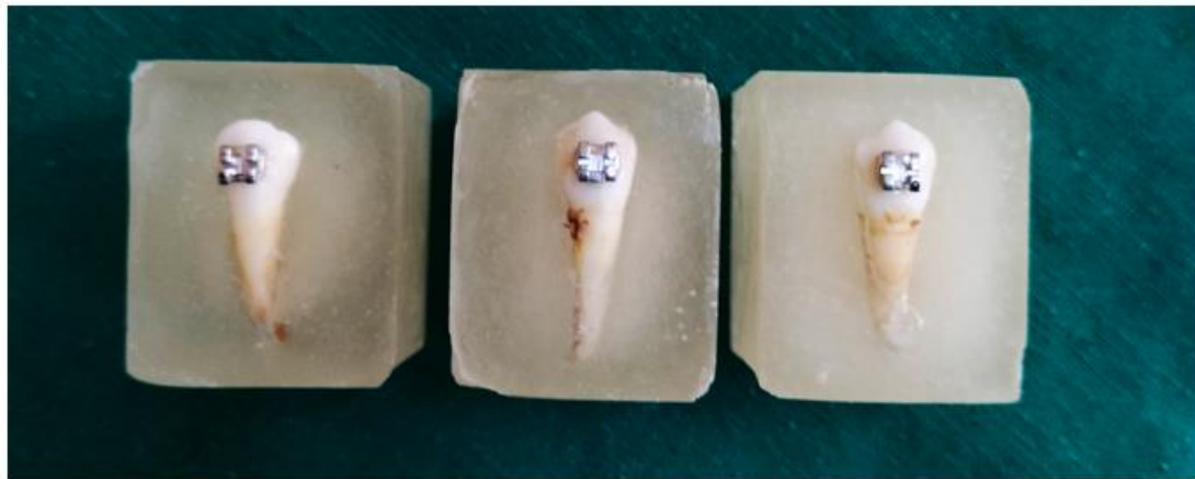
Fig. 1 Premolar teeth mounted in acrylic blocks for testing
