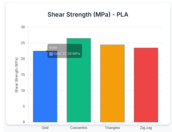
Fig 12.4:Graph for the Shear test values
