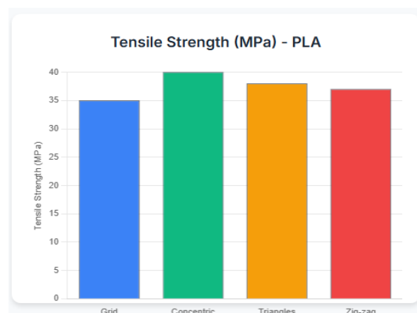
Fig 12.2:Graph for the Tensile test values
