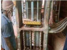
Figure 2.2.4 Block making (120kgf)
