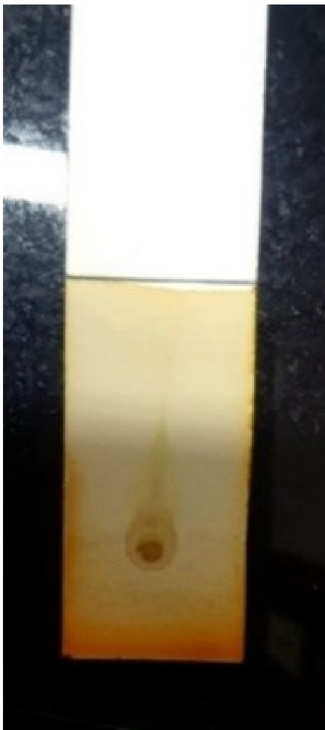
Figure 2. Thin-layer chromatographic profile of melanin extracted from Gallus gallus domesticus , displaying a single violet-colored spot with an R_f value of 0.67.
