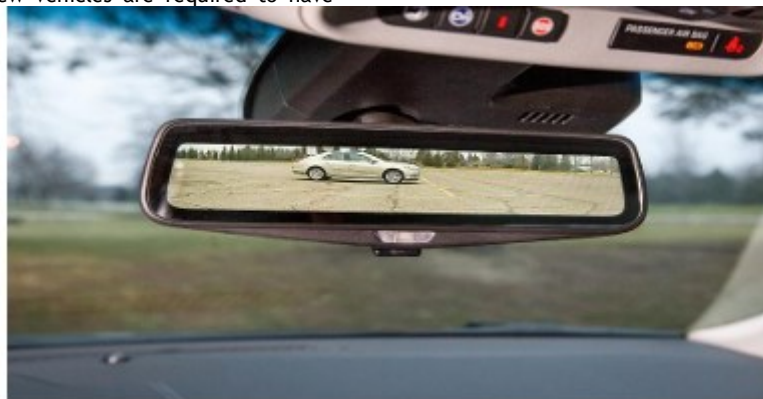
Fig-2: Camera Based Rear-View System
