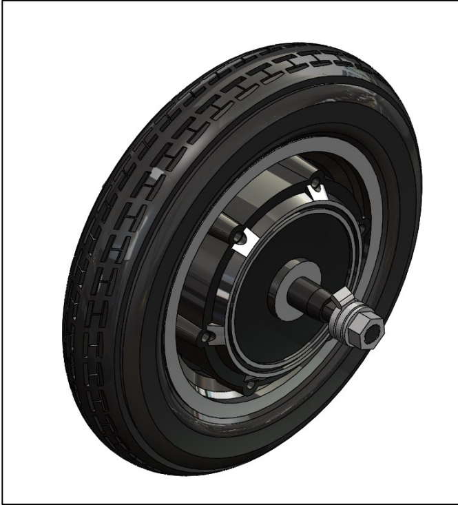
Fig. 5. CAD Model of the Wheel Hub Motor
