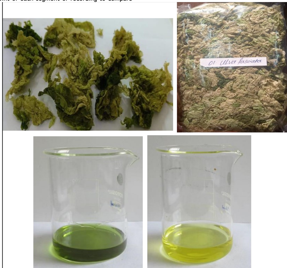
Figure 1. Fresh sample of Ulva fasciata collected and dried, made into powder, extracted with methanol and ethanol
