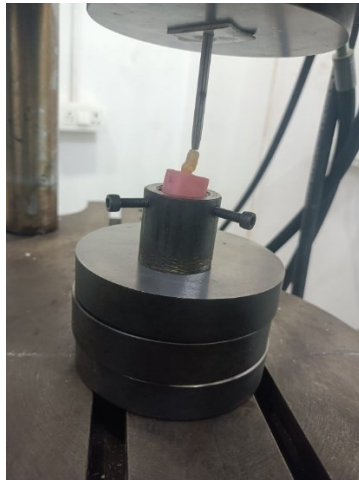
Figure 3. Sample under Universal Testing Machine.
