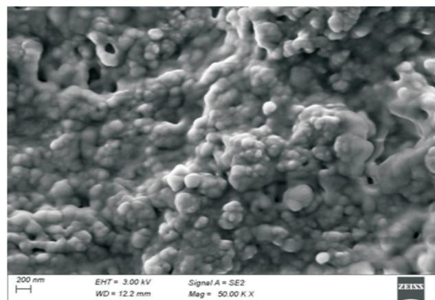
Figure 4. SEM image of synthesized CuNPs
