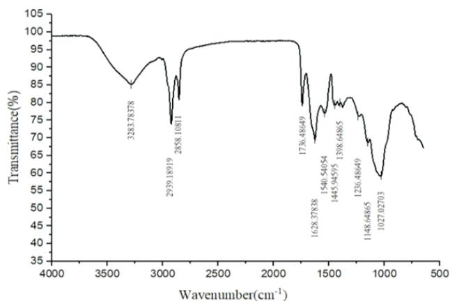
Figure 2. FTIR spectra of biosynthesized copper nanoparticles
