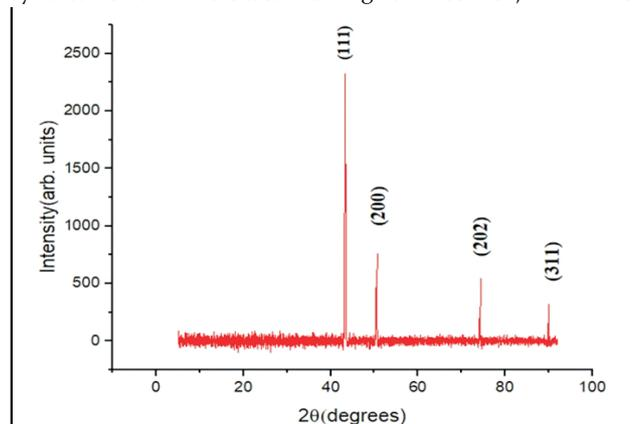
Figure 3. XRD analysis of copper nanoparticles
