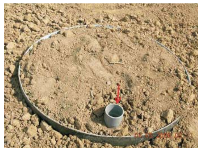
Figure 2(a): A cylindrical pit being dug for the fixation of lysimeter drum at the lysimeter site and (b) A freshly installed lysimeter filled up with field soil. Note the upper end of the observation well (arrow)
