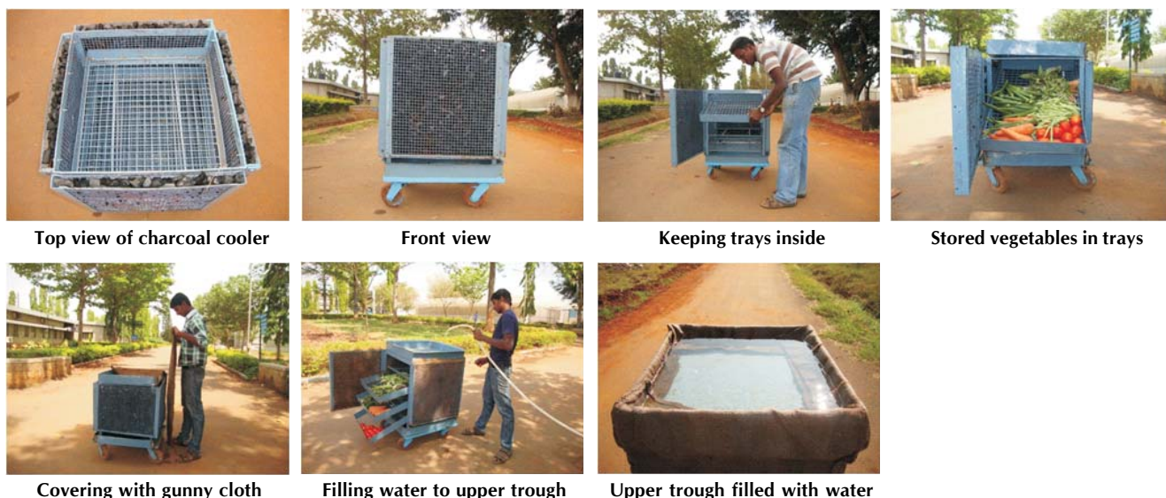
Plate 5: Stepwise operation of Charcoal cooler
