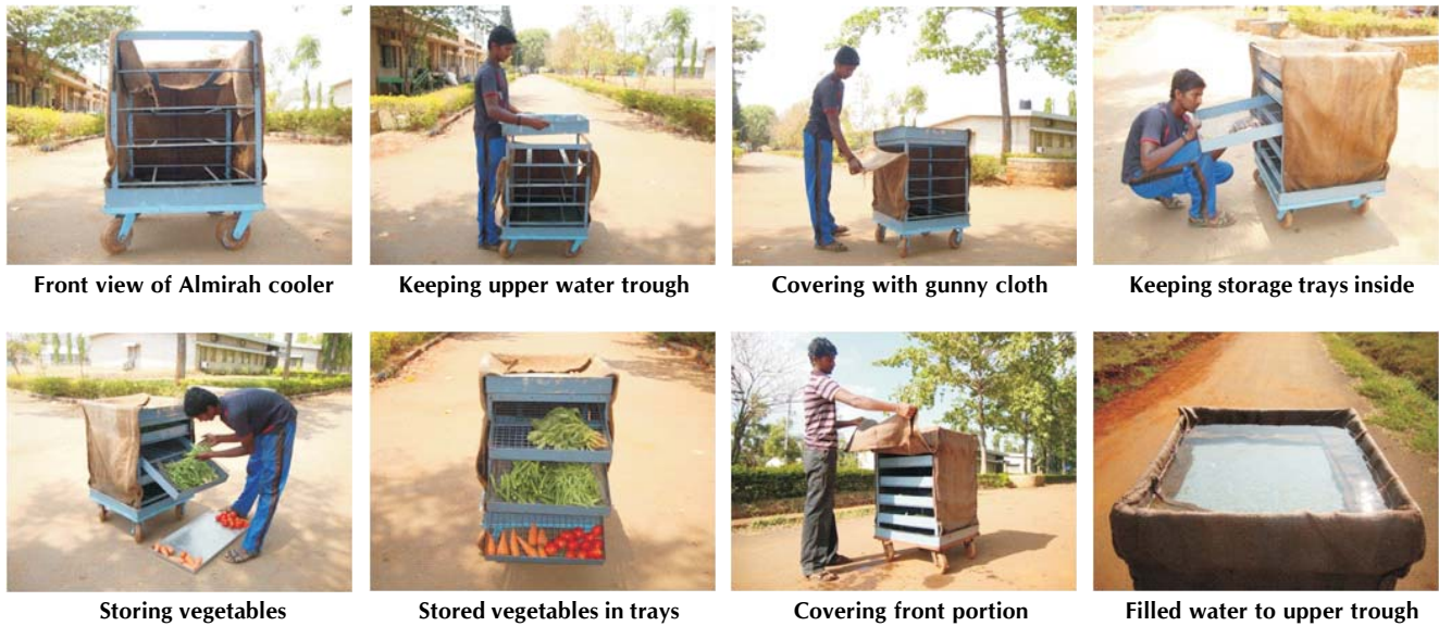
Plate 3. Step wise operation of Almirah cooler
