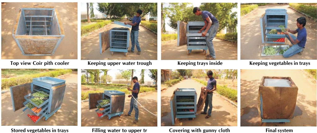
Plate 4 : Stepwise operation of Coir pith cooler
