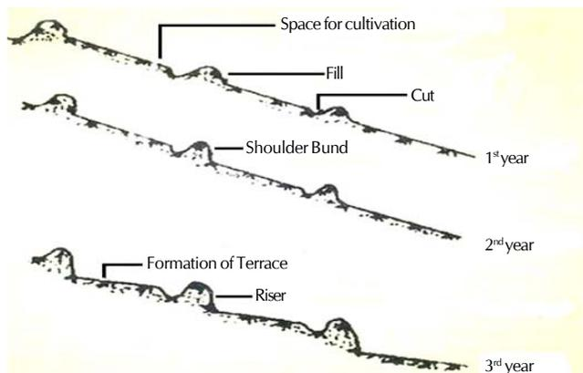
Figure 2: Contour bunding for slow conversion terraces
